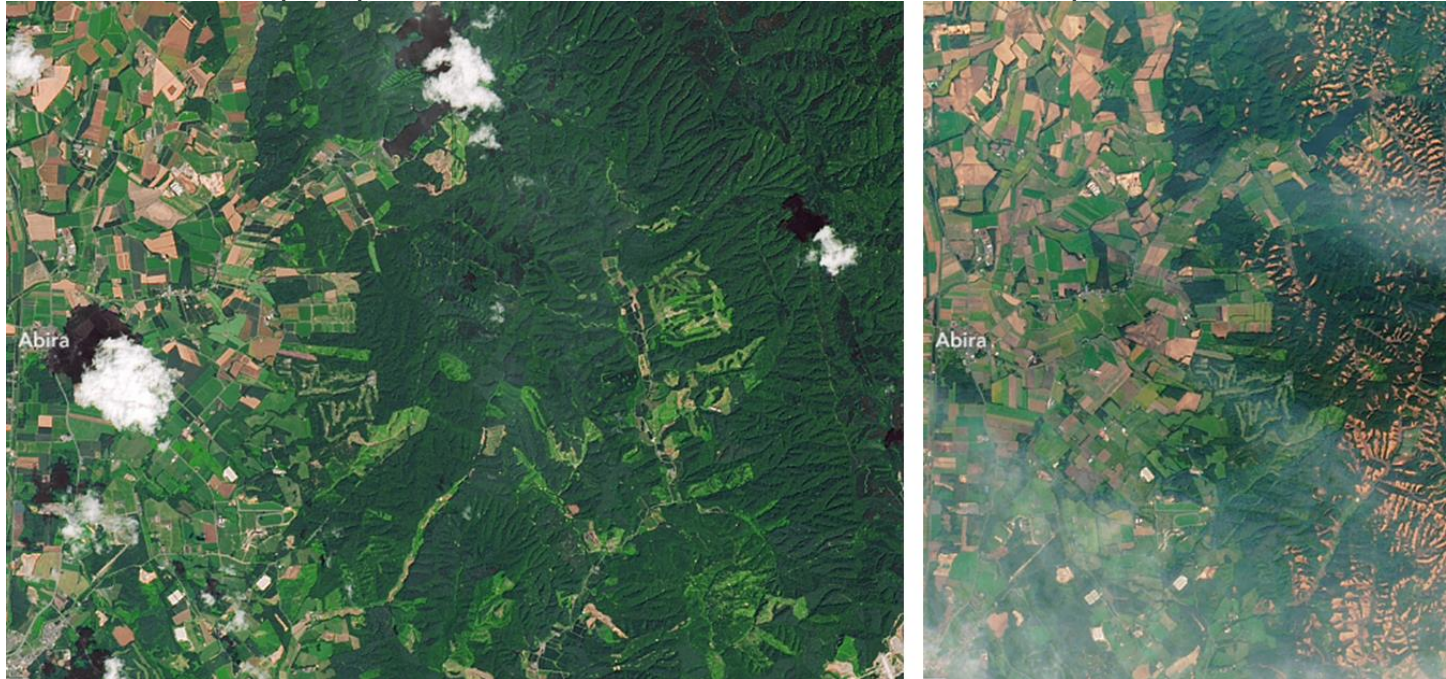
Figure 7.1.5 Slope failures in the Sapporo area of Japan following a typhoon (Sept. 4th, 2018) and earthquake (Sept. 6th, 2018) (Before and after Landsat 8 images: left: July 2017, right: September 2018). “Landslides in Hokkaido” by Lauren Dauphin, NASA Earth Observatory. Public domain.
