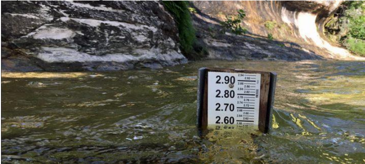
A stream gage showing water depth in the Colorado River. USGS. Public Domain
